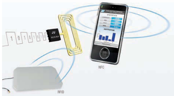
The M24LR64 wireless memory operates on the Android operating system, which connects an NFC-enabled smartphone to a prototype temperature recorder.
